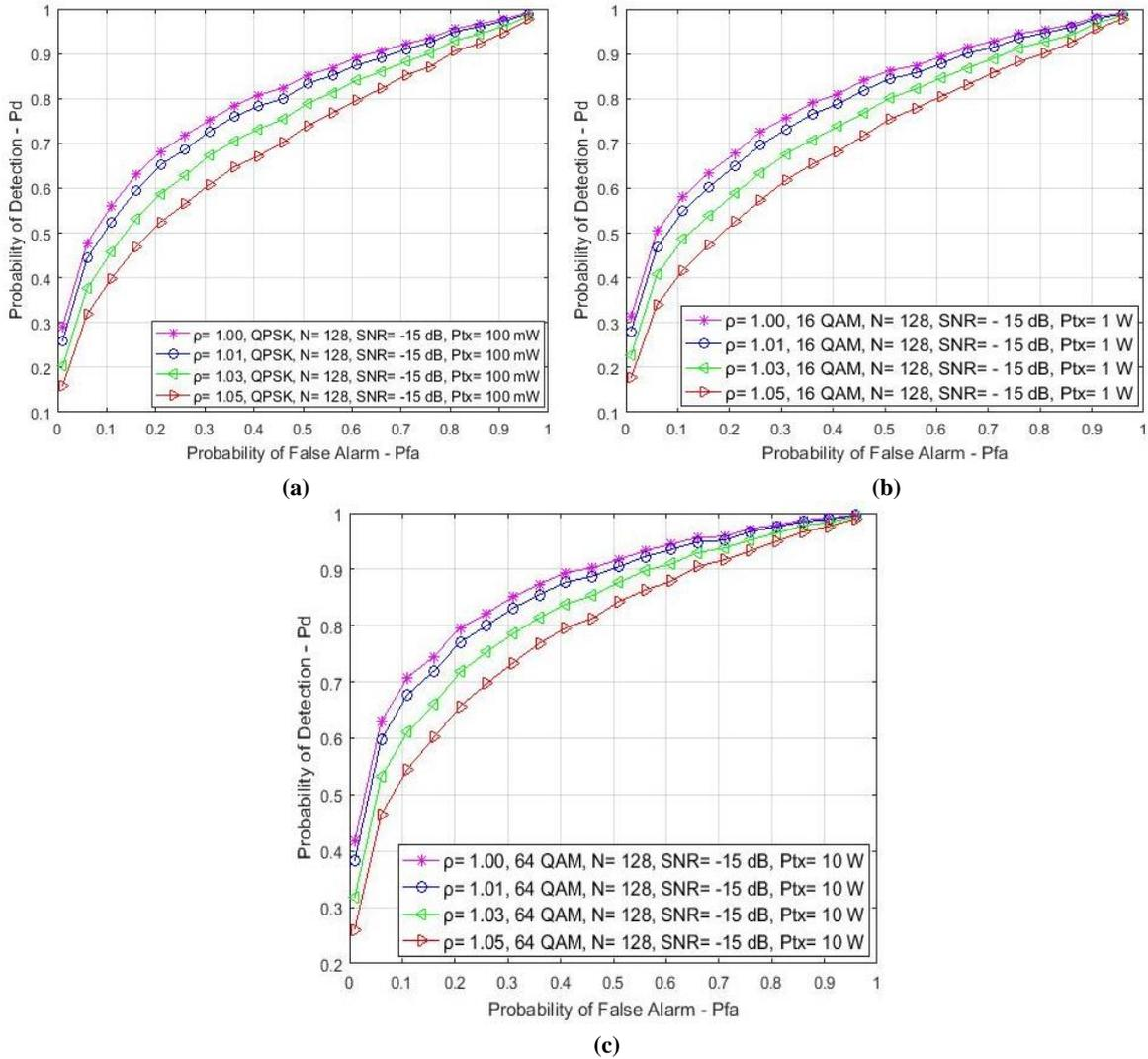
**Figure 3.** ROC curves for joint RA and MA OFDM systems impacted by different values of NU factors and transmitted with: (a) Tx power of 0.1 W and QPSK modulation; (b) Tx power of 1 W and 16-QAM modulation; (c) Tx power of 10 W and 64-QAM modulation
