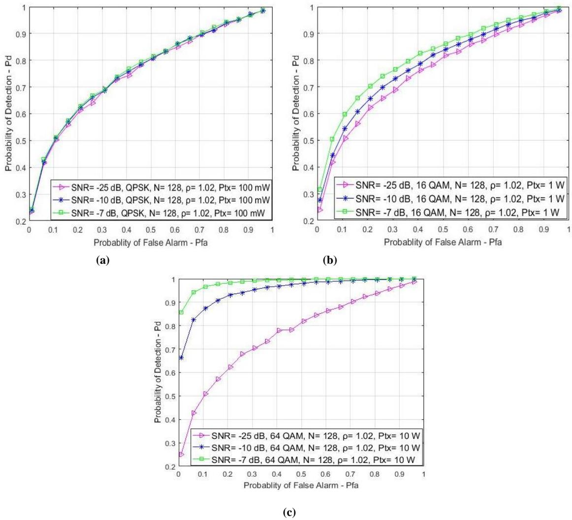
**Figure 7.** ROC curves for OFDM signals transmitted in joint RA and MA systems with Tx power equal to: (a) 0.1 W; (b) 1 W; (c) 10 W
