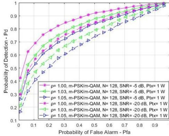
**Figure 2.** ROC curves for RA OFDM systems based on m-PSK/m-QAM modulations impacted by different values of NUs in the case of two different SNR levels
