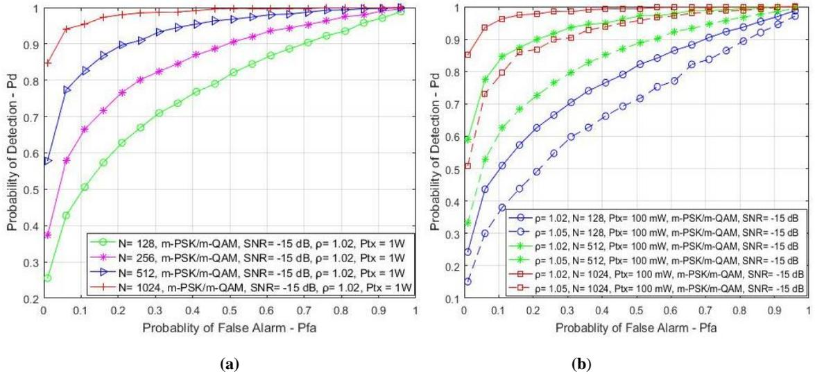
**Figure 9.** ROC curves for m-PSK/m-QAM modulated signals transmitted with fixed Tx power and detected with different number of samples for: (a) equal NU ( $\rho=1.02$ ); (b) two different levels of NUs ( $\rho=1.02$ ,  $\rho=1.05$ )
