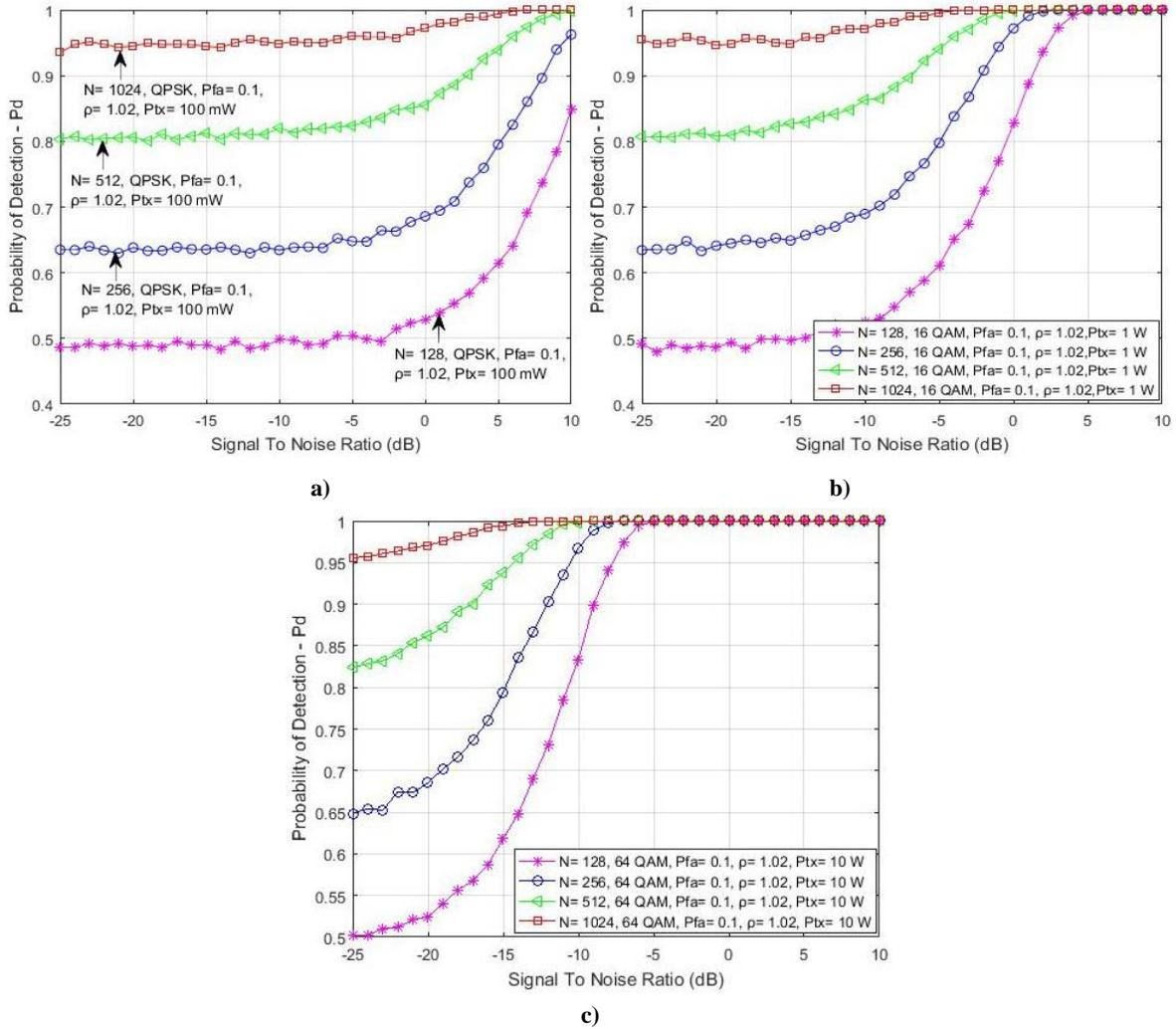
**Figure 11.** Impact of SNR and number of samples on the probability of detection for joint RA and MA system of OFDM signal transmitted at: (a) 0.1 W; (b) 1 W; (c) 10 W
