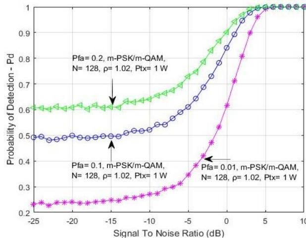
**Figure 12.** Impact of SNR on the probability of detection for RA OFDM systems with different probabilities of false alarm
