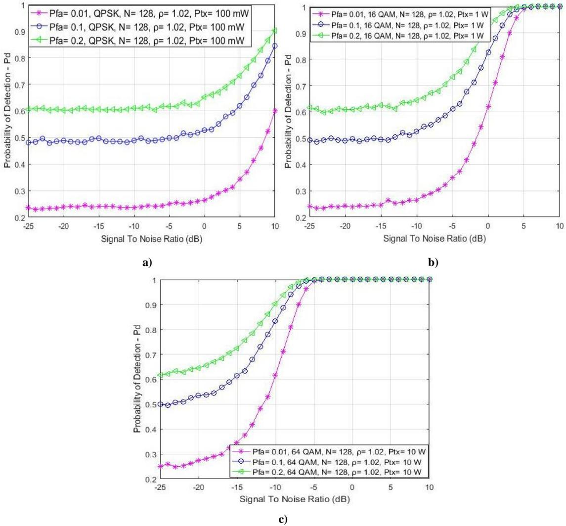
**Figure 13.** Impact of SNR and the probability of false alarm on the probability of detection for joint RA and MA OFDM systems transmitting at: (a) 0.1 W; (b) 1 W; (c) 10 W
