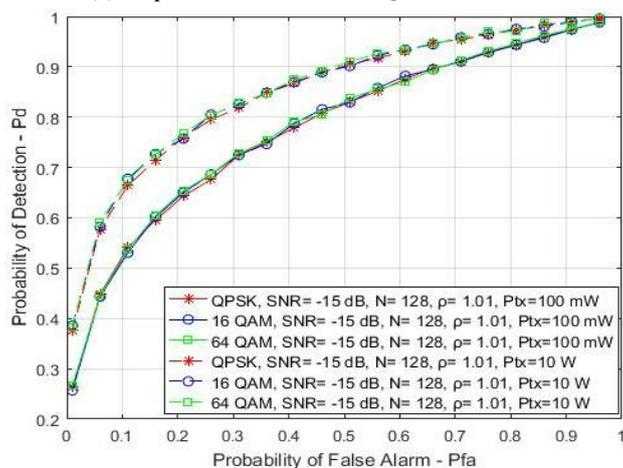
**Figure 4.** ROC curves for MA systems impacted by equal NUs for different Tx powers and OFDM modulations
