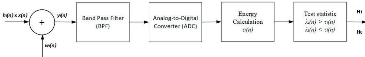
**Figure 1.** Block diagram of the energy detection technique
