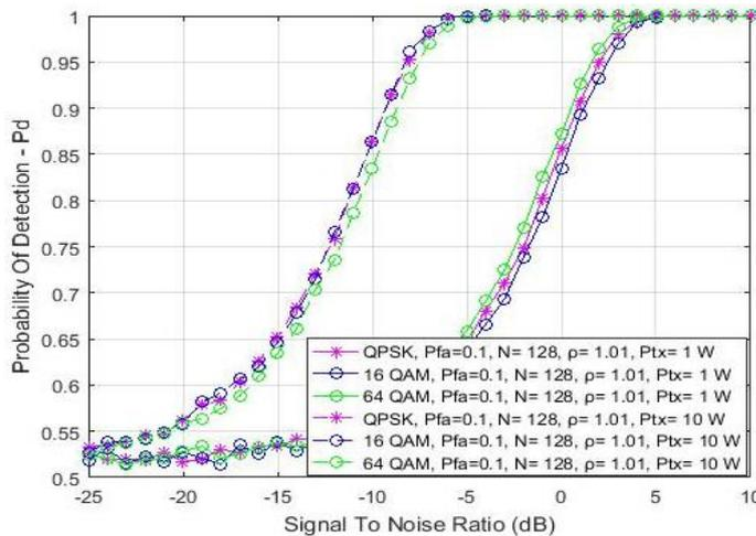
**Figure 8.** Probability of detection vs. SNR for MA OFDM system transmitting at two different Tx power levels
