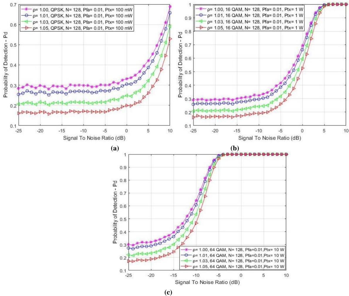
**Figure 6.** Influence of SNR on the probability of detection for OFDM signals impacted with different NUs and transmitted with Tx power of: (a) 0.1 W; (b) 1 W; (c) 10 W
