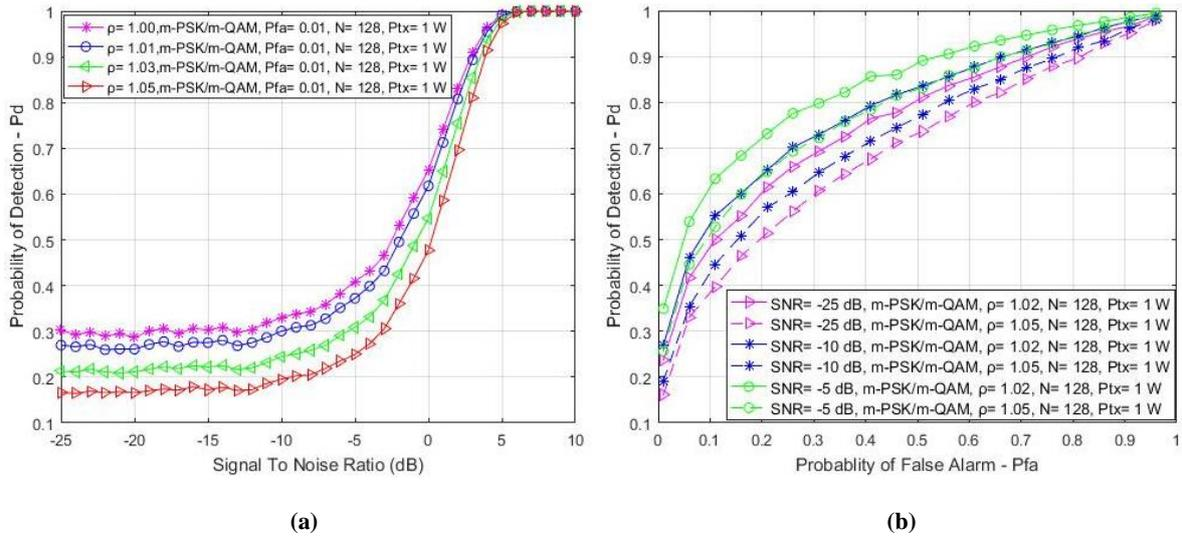
**Figure 5.** (a) SNR vs. probability of detection for OFDM signals impacted by different NUs in RA systems; (b) ROC curves for different values of SNR for an RA OFDM system transmitting signals modulated with m-PSK/m-QAM modulations and impacted by two different NU factors
